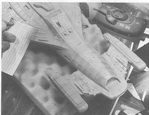
Weathered panels being sprayed onto the upper Primary Hull. Note pattern on Nacelles and Shuttle Landing Platform.
